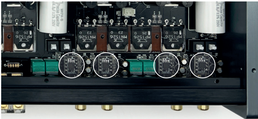
MUSES8820 Mounted on PCB to fit the socket
