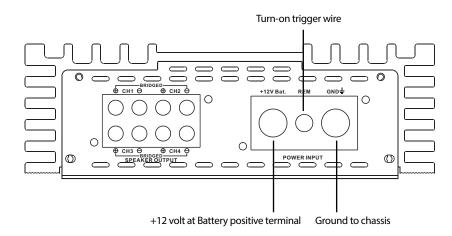
Note: The Z-Series AP amplifiers have terminals that do not require connectors. You simply insert a bare portion of wire and tighten the connection. As the wire conforms to the connector the connection can loosen. You should re-tighten the connection after about a week.
