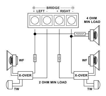
A 3-Way hookup requires a coil on the woofer and capacitors on the highs to act as a crossover and maintain correct impedance. Consult the speaker manufacturer for correct cap and coil values.
