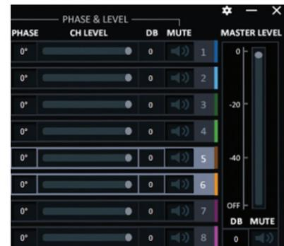
There are a number of systems for checking System Phase. If the systems speakers are not all in phase there will be issues you can not fix by tuning. You can see the section on System Phasing to see one method of Phase checking. The MUTE buttons allow you to turn off any speakers that you do not want to hear while you are tuning other speakers. You will also find a master level control here and a system MUTE button.
