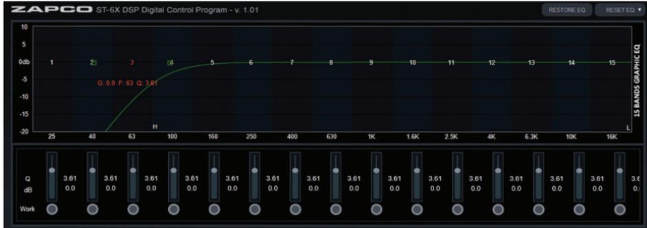
Here are 15 bands of parametric equalization for each output channel and you can vary Frequency, Gain, and Q (the shape of the adjustment) for each band in several ways. Frequency: Each band is numbered. You can simply click onto a band button and drag it to where you want it. When you click onto a band there is a “Heads-up display” of the frequency, gain, and Q of the band. Any band that has been adjusted from 0dB is highlighted by the green dot under the band’s slider.
