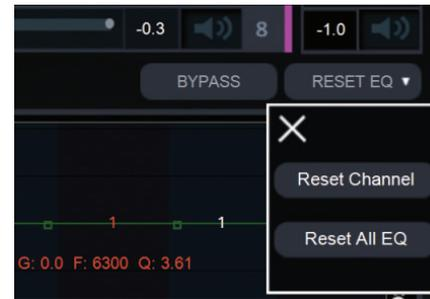
To aid the tuning process you can temporarily bypass a channels equalization. You can also reset one channel or reset all channel to default positions with no equalization.
