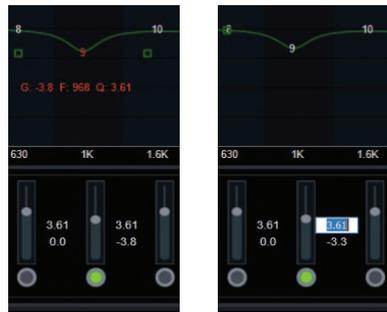
Left: Band # shows in Red, as do the Gain, Freq., and Q. The green squares show the width (Q) of the filter. Right: you can click into the Gain or Q value box of any band and adjust using the up/down arrow keys.
