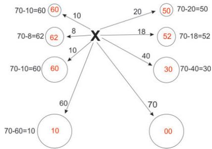
In this example, the longest speaker distance is 70" so we subtract each of the other speakers from 70 and enter the results in the Delay chart.
