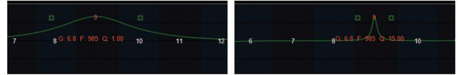
**Q Setting:** Q can be set as above using the keyboard arrows. You can also make rough adjustments by dragging one of the green boxes in the EQ graph to make Q wider or narrower to affect a smaller or larger group of frequencies with your EQ adjustment.
